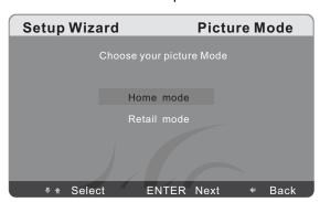
4 Press ▲ or ▼ to select the Home Mode or Retail Mode, then press ENTER. Home Mode reduces the TV's total power consumption. The Tuner Mode screen opens.
